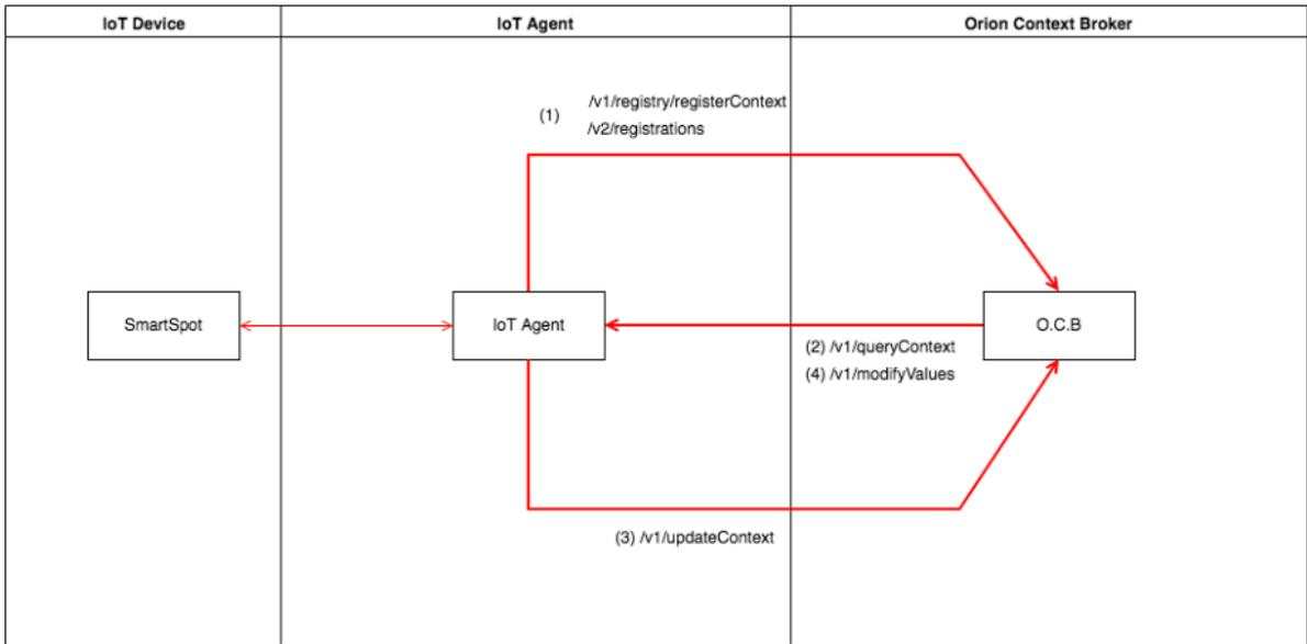
Figure 5 – Fogflow IoTAgent Communication Requirements
