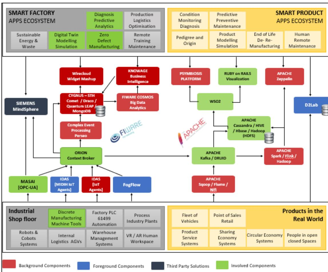
Figure 15 – Data flow for the Smart Factory Scenario (NECO Use Case)
