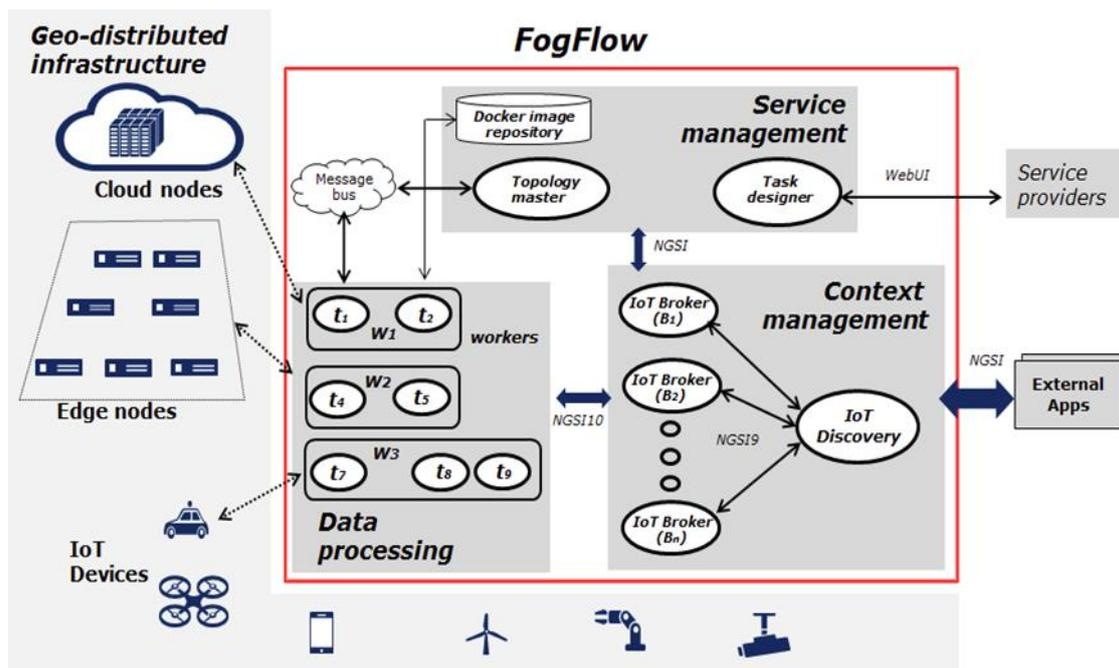
Figure 3 – General view of the Fog Flow framework
