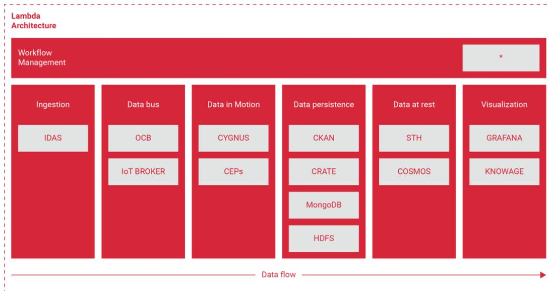
**Figure 20 – FIWARE Pipeline for Industrial IoT and Analytics Platform**
