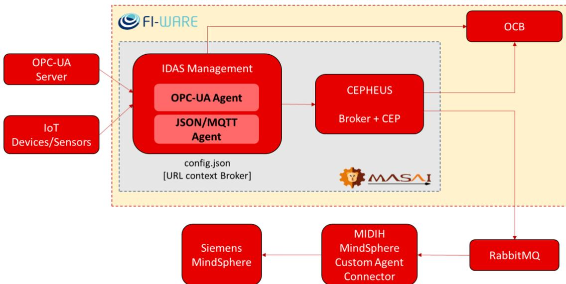
Figure 4 – MIDIH OPC-UA Connector for Siemens MindSphere Architecture
