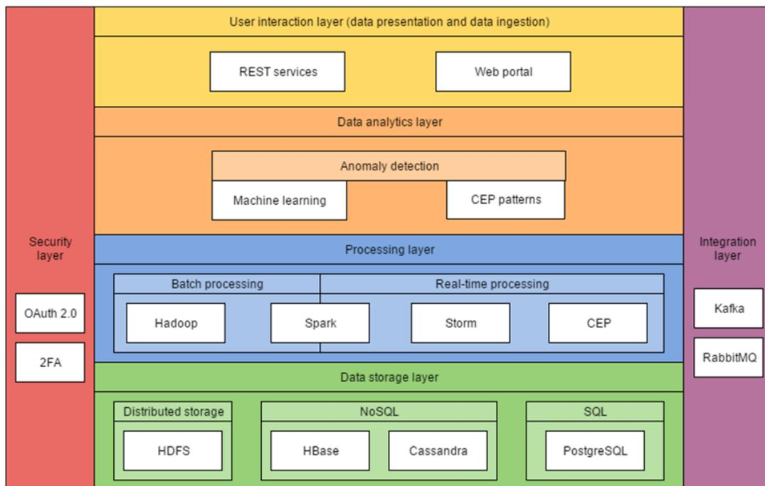
Figure 7 – D2lab conceptual architecture
