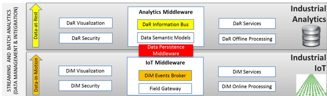
**Figure 10. MIDIH Data Analytics Framework for data-in-motion and data-at-rest**
