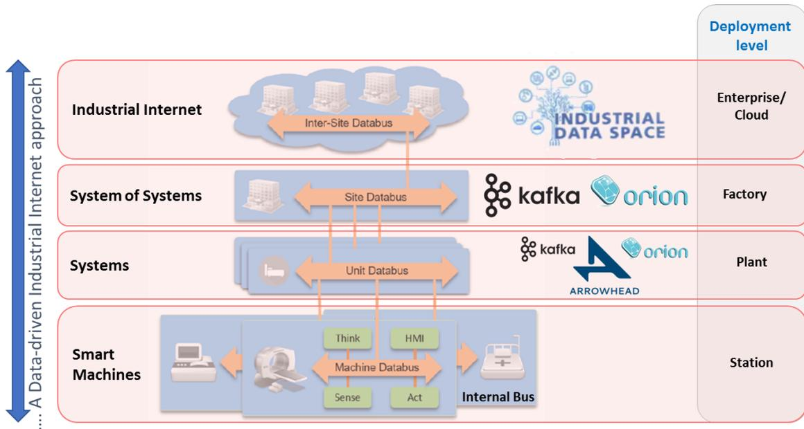
**Figure 9. MIDIH Reference Implementation of the Layered Databus pattern**
